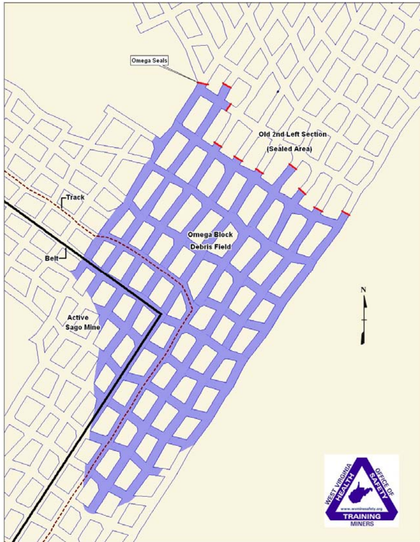
MAP 2: This illustration shows the approximate distance and symmetry of the debris field created by the ten (10) destroyed Omega seals.
